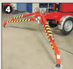
4 Hydraulic support legs allow a quick and safe set up even on sloping ground.
